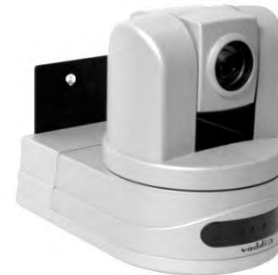
Completed CONCEAL Wall Mount Camera Bracket Installation
