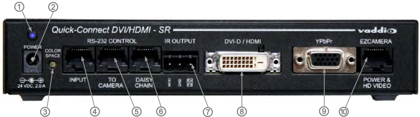
Image: Rear Panel Connectors and Features
