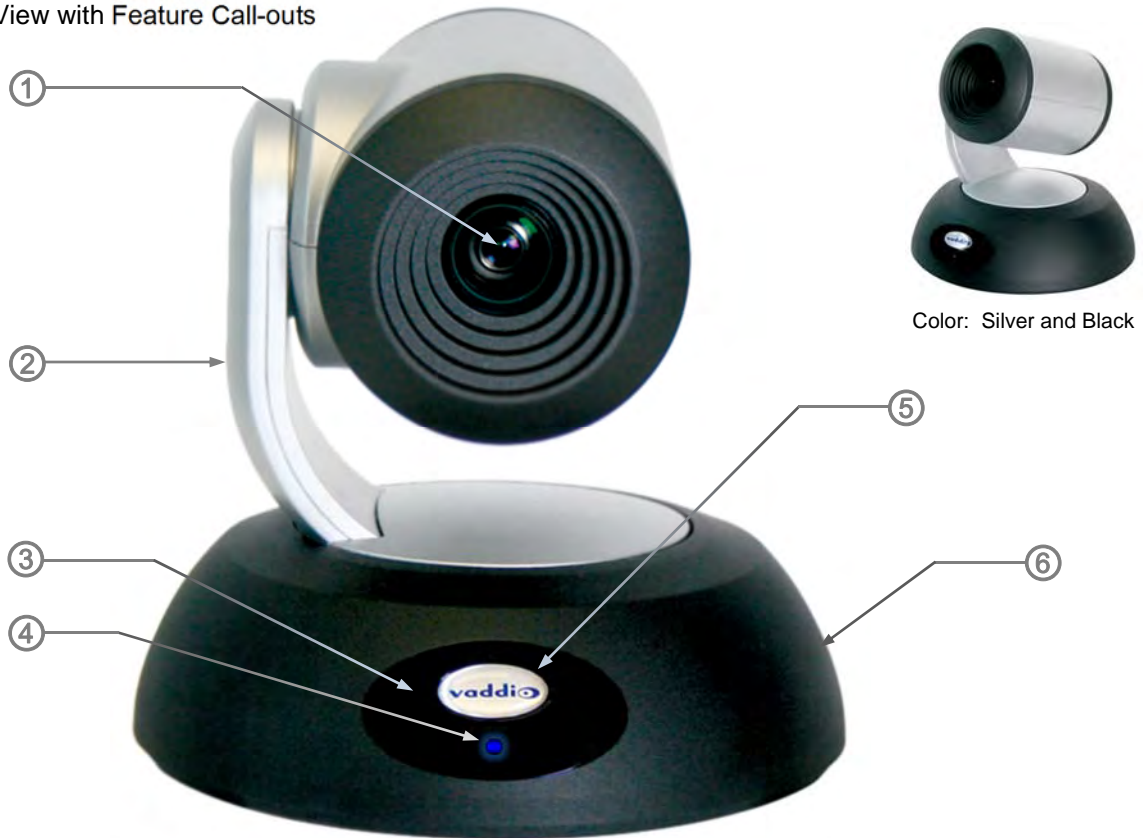
Image: RoboSHOT 12 Camera Camera Front View with Feature Call-outs
