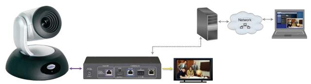
The OneLINK™ HDMI extension module is not required; the camera can be connected directly to the network.
