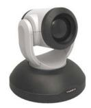
The camera optics shall feature a 12x optical zoom lens with seamless transition to 1.67x digital zoom, for a total zoom range of 20x. The camera shall use a 1/2.3-type, high-speed, low noise, back-illuminated CMOS sensor with 9.03 total megapixels, producing native 2160p/30 (3840 x 2160) video images without scaling.
