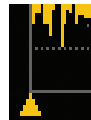
Pre/Post-Trigger Indicator appears at the edge of the grid when trigger point is no-longer visible.
