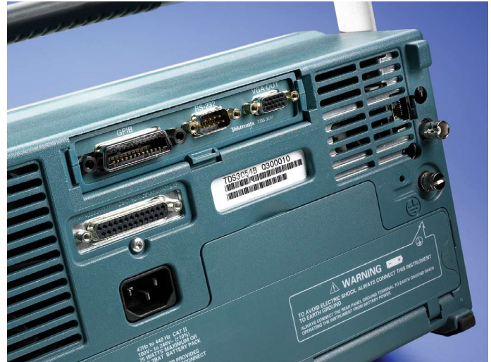
Figure 53. Today's oscilloscopes provide a wide array of communications interfaces, such as a standard Centronics port and optional Ethernet/RS-232, GPIB/RS-232, and VGA/RS-232 modules. There is even a USB port (not shown) on the front panel.
