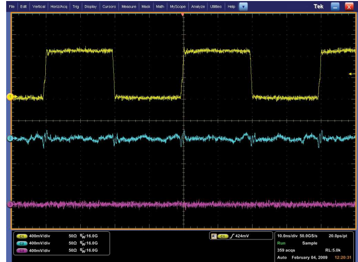
Figure 42. Differential probes can separate common-mode noise from the signal content of interest in today's fast, low-voltage applications - especially important as digital signals continue to fall below typical noise thresholds found in integrated circuits.
