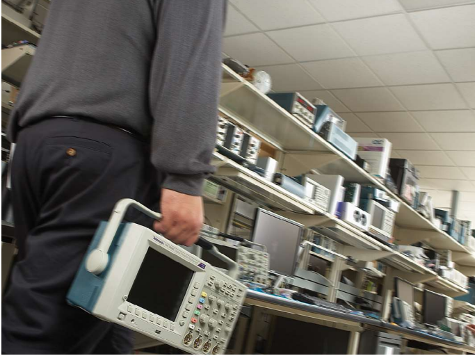
Figure 63. The portability of many oscilloscopes makes the instrument efficient in many operating environments.
