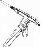
Freehand Probe Holder The FreeHand lets you focus on the oscilloscope screen instead of on maintaining contact to multiple test points. It allows the user to concentrate on what is really important – the waveform.
