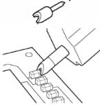
The crescent shape of this tip is designed to fit tightly on capacitors, resistors, transistors and other surface mount components with discrete leads. Fits in either probe socket.
