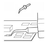
The Bent Tip is made out of titanium, this tip is ideal for situations that require the user to hold the probe parallel to the circuit board under test. Also gives you more control when holding the probe like a pencil. Fits in either probe socket. (PACC-PT005)
