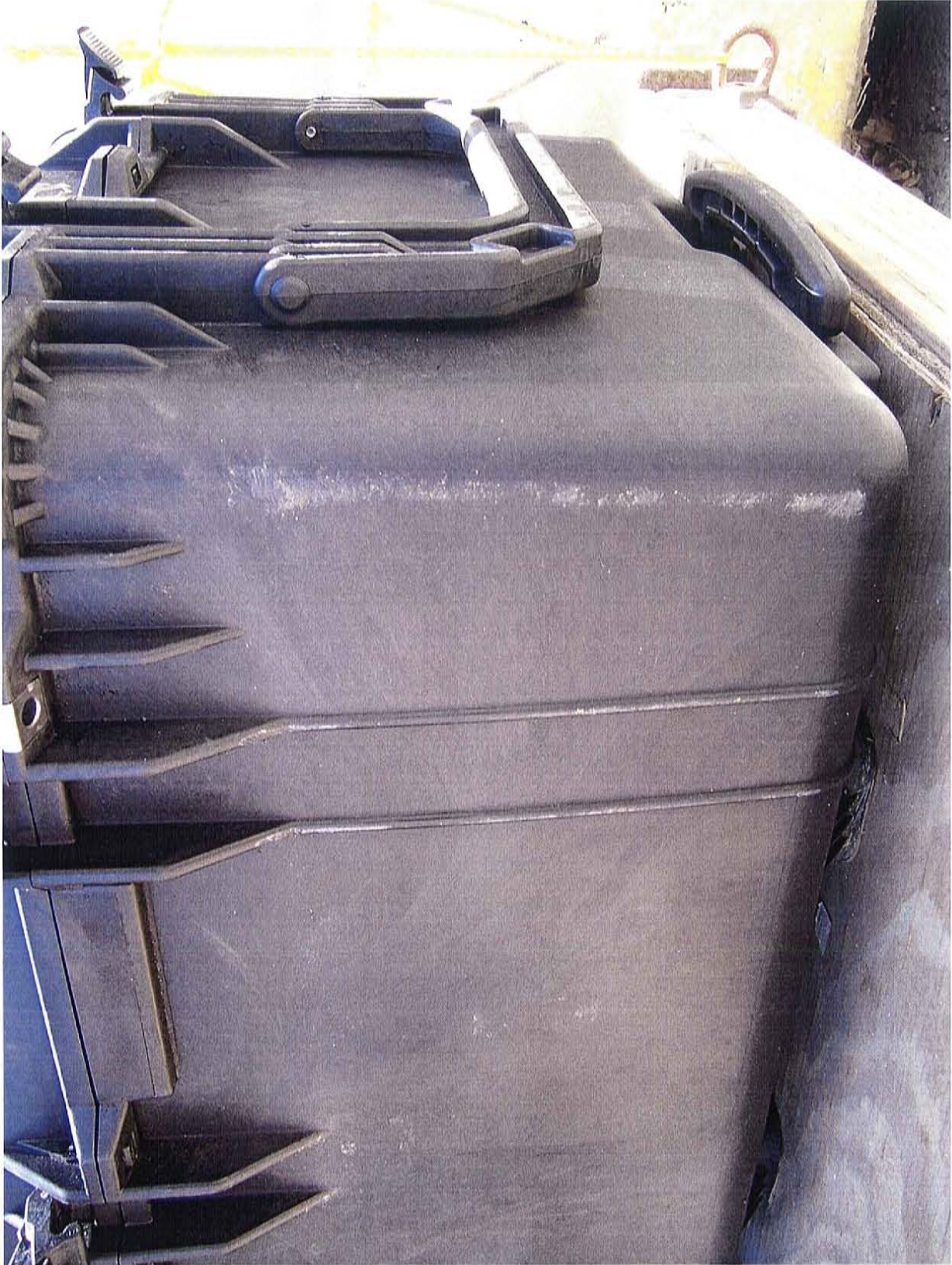
Photograph 13 Post Impact Test – Minor Scratches on Container Surface
