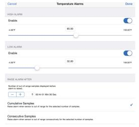
5. Enable the Low Alarm if you want an alarm to trip when the sensor reading falls below the low alarm value. Drag the slider to the reading that will trip the alarm or tap the value field and type a specific reading. In the example, an alarm is configured to trip when the temperature falls below 32°F.
