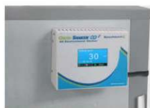
Remote controller adjusts shaker settings from outside of the chamber and magnetically attaches to most incubators
