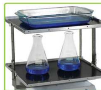
Add/remove platforms to create the ideal capacity and spacing for your application (up to 8 1/4 in. clearance)
