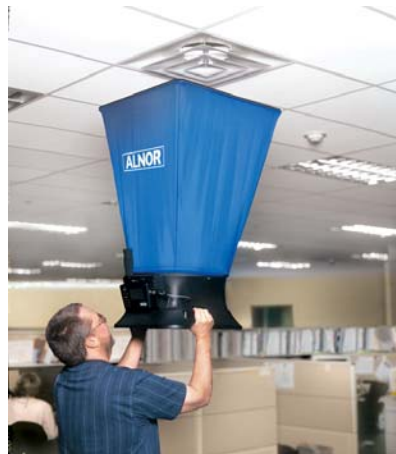
EBT721 measuring a supply diffuser
