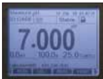
Reading turns solid when stable.
