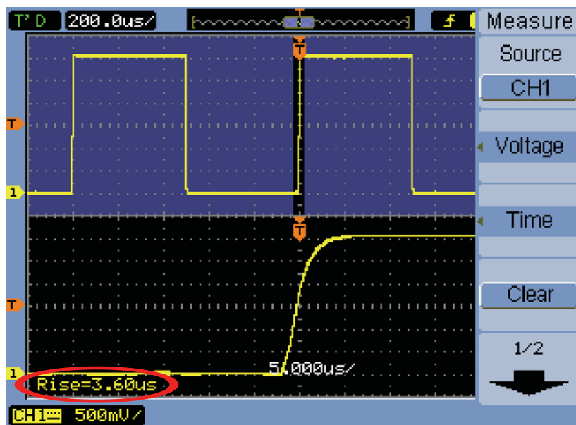
Figure 31 Making an accurate “gated” rise time measurement using the scope’s zoom mode
