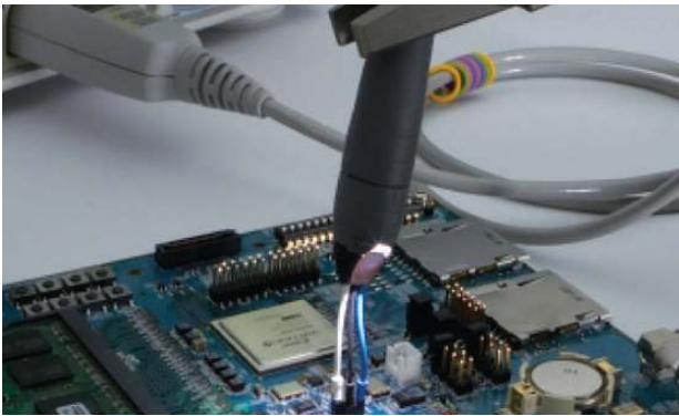
InfiniiMode probe with either socketed tip or solder-in tip allows convenient measurements of differential, SE and CM signals with a single probe. Probe head light is built in.
