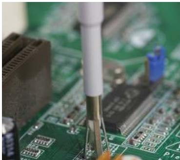
N2885A PCB adapter kit for N2870A Series passive probes (probe not included)
