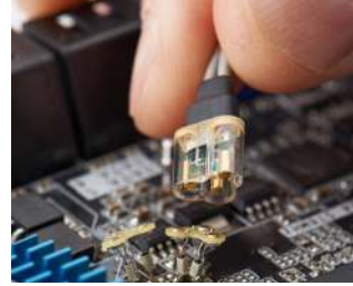
N2848A QuickTip head with N2849A QuickTip tips
