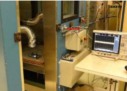
N2797A for testing devices in environmental chambers.
