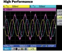
Automatically displays measurements for both isolated channels from your choice of 19 measurement types.
