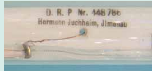
Figure 1: Original contact thermometer from year 1926, German Reich Patent (detail).
