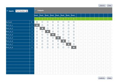
Select the radio button at the corresponding intersection of the input/ output ports you want to connect, to connect each input source to an output display.
