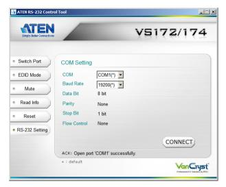
The controller's serial port should be configured as follows:
