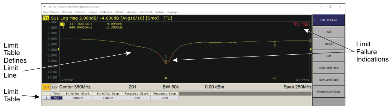
Figure 74 Limit test schematic
