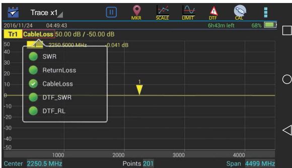
Figure 30 Selecting Cable Loss Measurement
