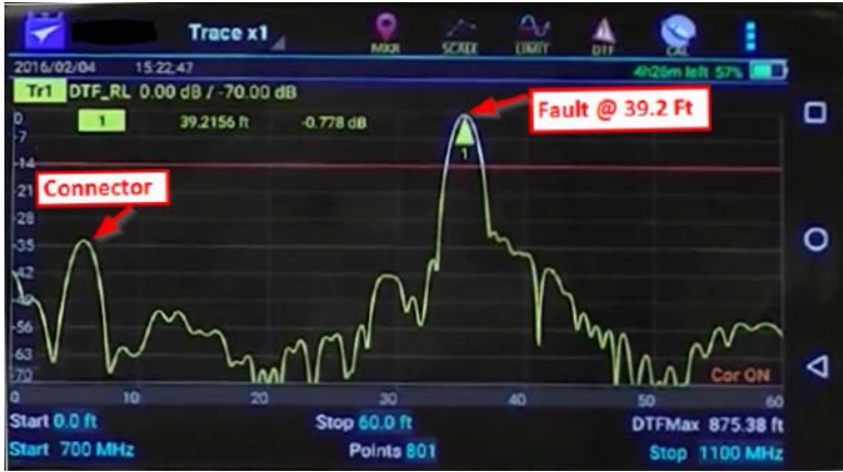
Figure 1 Typical Fault Location Measurement
