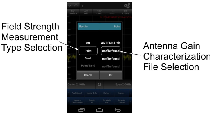
Figure 19 Field Strength Measurement
