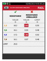
But there's a catch. While ISO/IEC 11801:2010 provides DC Resistance Unbalance test limits for the Channel and Permanent Link definitions, ANSI/TIA-568-C.2 only provides test limits for the Channel definition.
