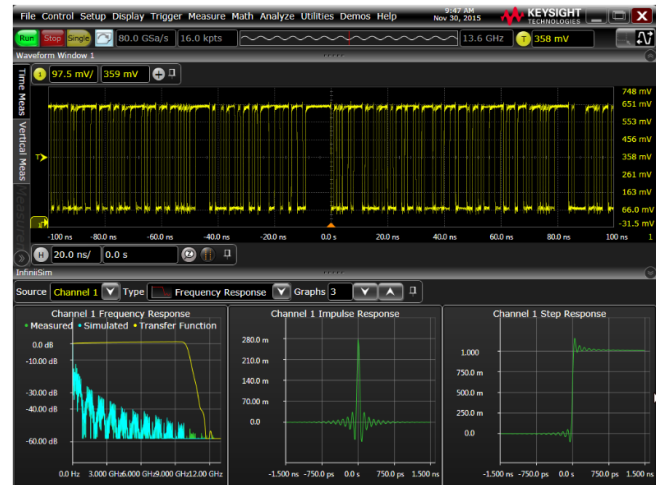
Figure 1. Results from InfiniiSim showing what a signal would look like with no cable between the DUT and the oscilloscope.
