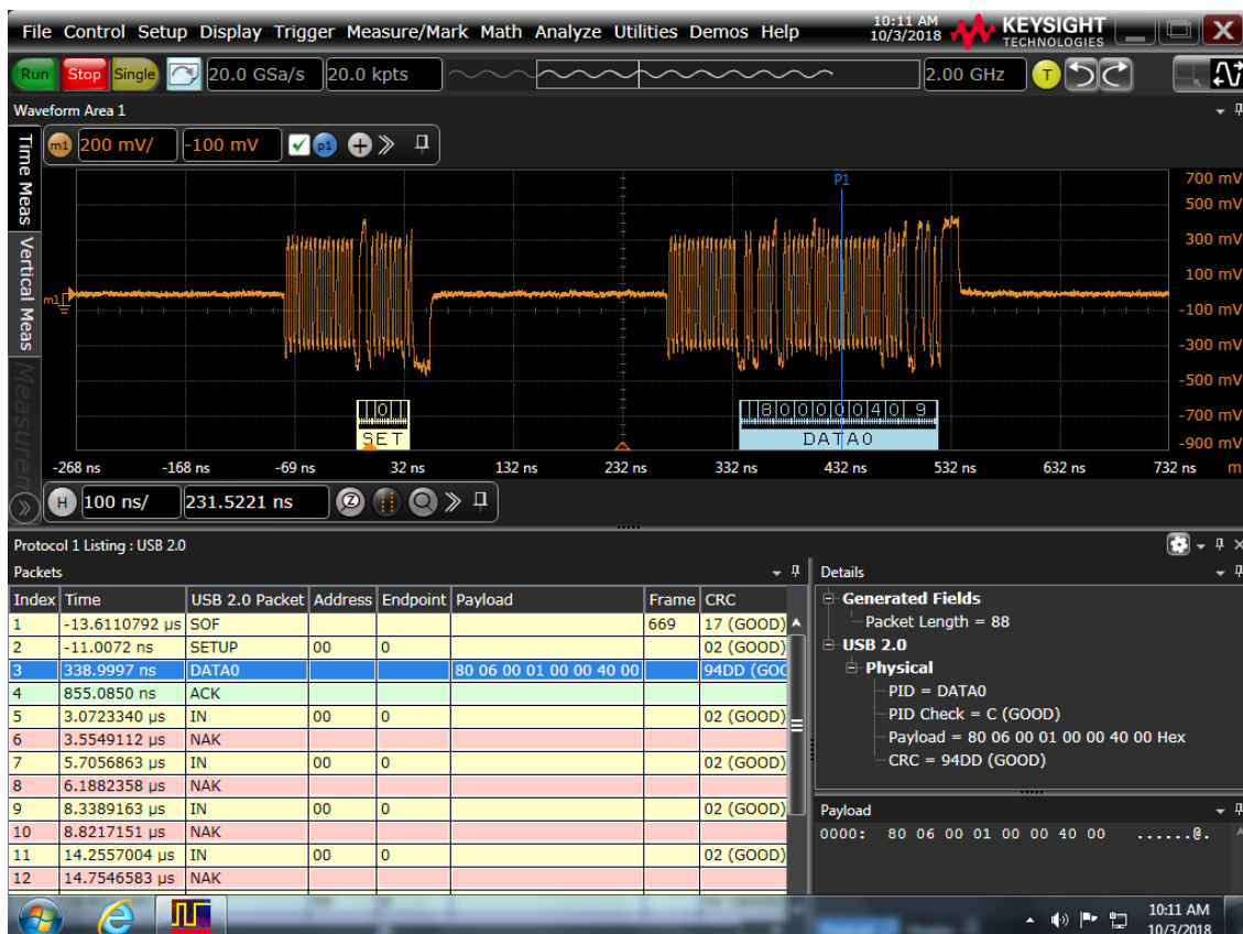
Figure 2. USB high-speed trigger and decode, with protocol lister and detailed packet view.
