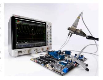
Hardware-based triggering ensures that the scope never misses a trigger event when armed. This hardware takes signals acquired using either scope or digital channels and reconstructs protocol frames. It then inspects these protocol frames against specified protocol-level trigger conditions and triggers when the condition is met.
