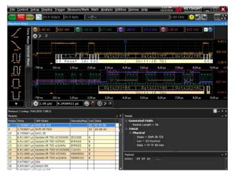
standard BSDL files, displays JTAG protocol in real time, and flags certain types of error conditions. Signals must be probed at the periphery of the scan chain and cannot be probed in the middle of the scan chain.
