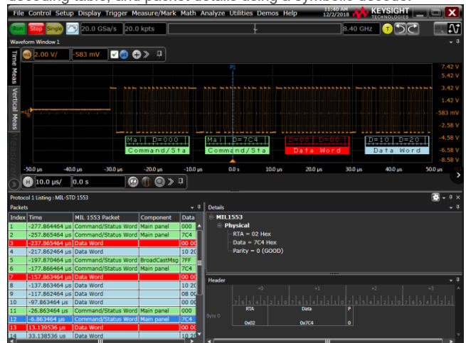
Protocol decoding of MIL-STD-1553 showing a real time trace, protocol decoding table, and packet details using a symbolic decode.
