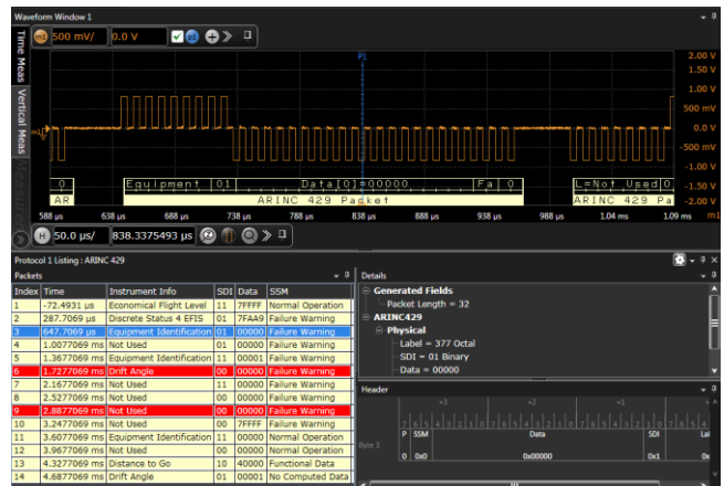
Protocol decoding of ARINC 429 showing a real time trace, protocol decoding table, and packet details using a symbolic decode.
