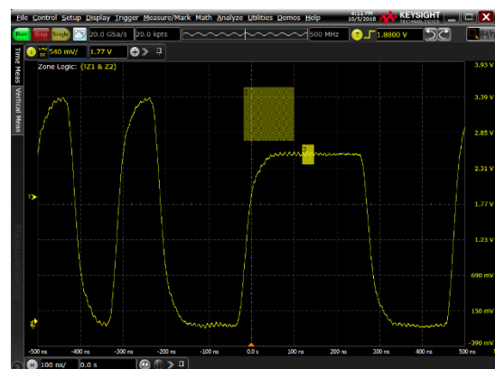
Figure 3. InfiniiScan zone qualification used to isolate a two bit wide runt.
