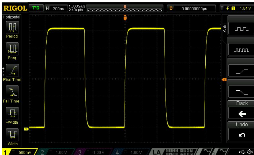
Rolling Plot of 1 MHz Signal from DSK Board
