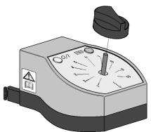
9.3.2. Remove and retain the regulator spindle locknut and shakeproof washer.
