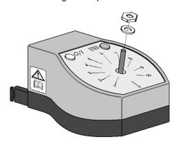
9.3.3. Turn the controller up-side down and remove the two fixing screws retaining the base. Lift the base off.
