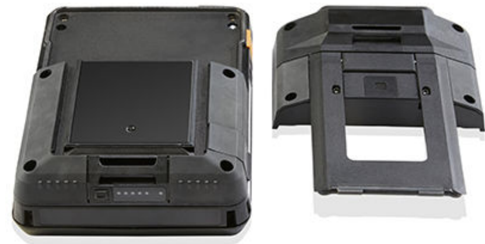
Figure 2-7: Trex unit with the communication module removed
