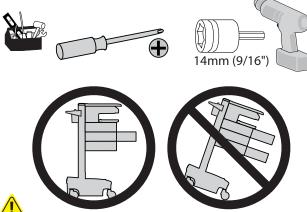
**CAUTION:** Close worksurface before opening drawers. Open only one drawer at a time. Do Not push cart when drawers or worksurface are open. Failure to follow these instructions may cause the cart to be unstable.
