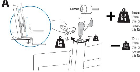
Increase Lift Strength If the mounted weight is too heavy or this product does not stay up when raised, then you'll need to increase Lift Strength:
