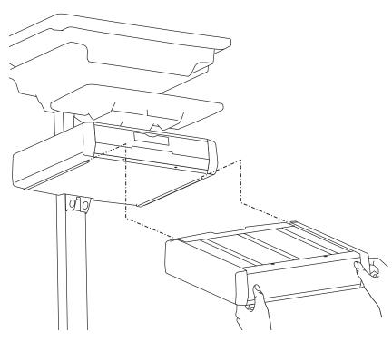
Plug the cable on the bottom drawer into the jack on the bottom of the drawer above it.
