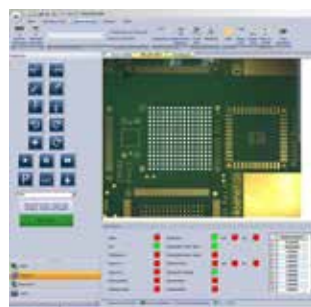
Superimposing of component and target position
