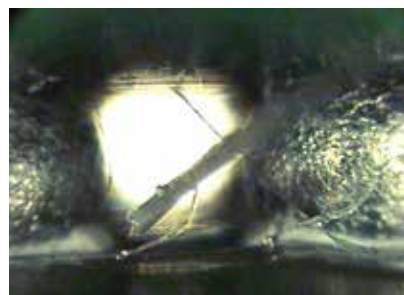
BGA: contamination (fibre)
