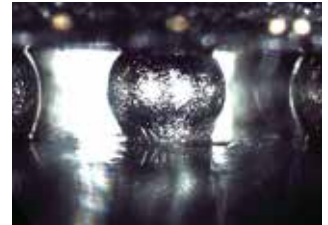
PBGA - cold joint: insufficient heat
