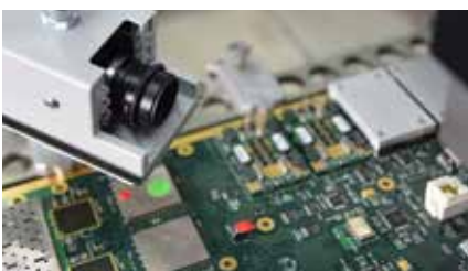
Live process monitoring on the HR 600 XL
