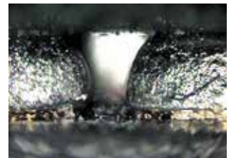
PBGA - scaling: insufficient heat
