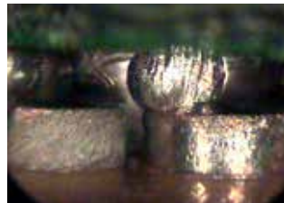
BGA - piggy back: bad alignment
