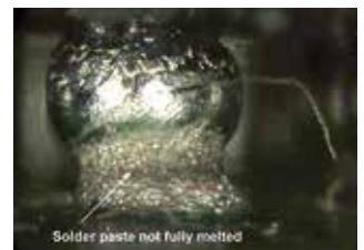
PBGA - scaling: insufficient heat
