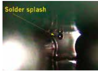
BGA: via hole solder splash
