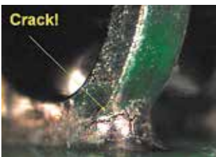
Lead-free PLCC: micro crack
