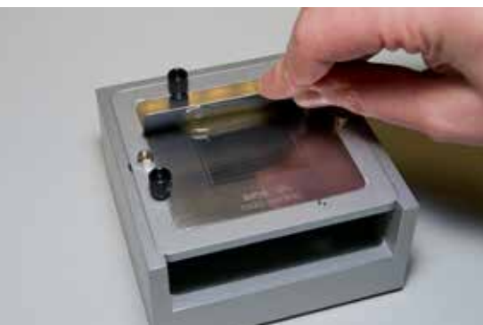
Flux deposition in the dip stencil
