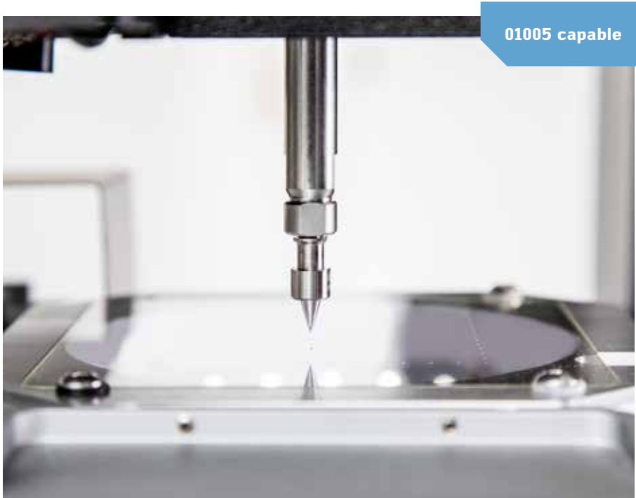
Automatic pick-up of a 01005 chip
