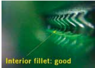
PLCC - interior fillet inspection
