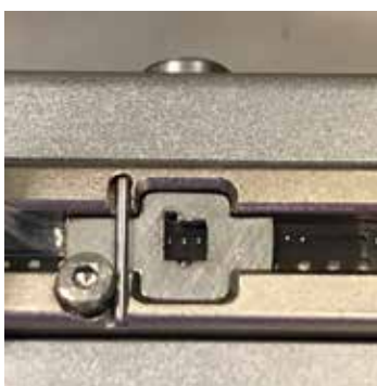
Provision of 01005 components with a tape feeder
