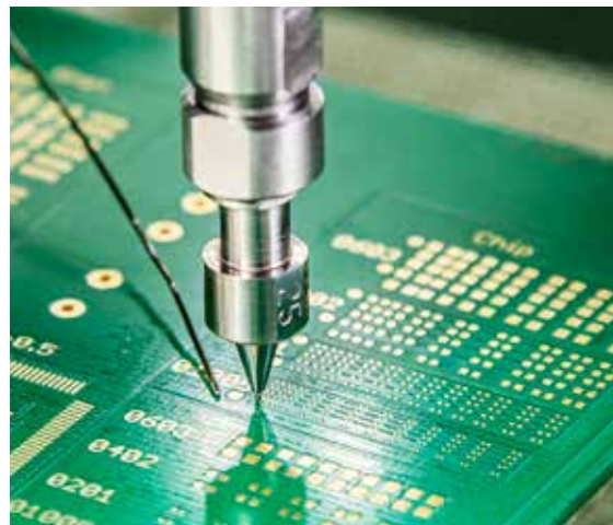
Automatic pick-up of a 01005 chip
