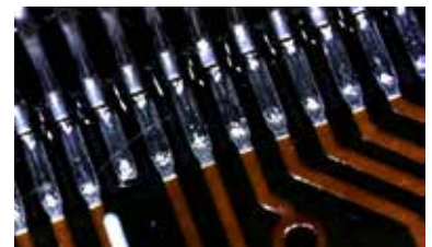
QFP solder joints – taken with the Ersa MOBILE SCOPE MACROZOOM optical head
