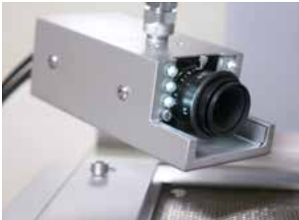
Reflow Process Camera (RPC) on the HR 550
