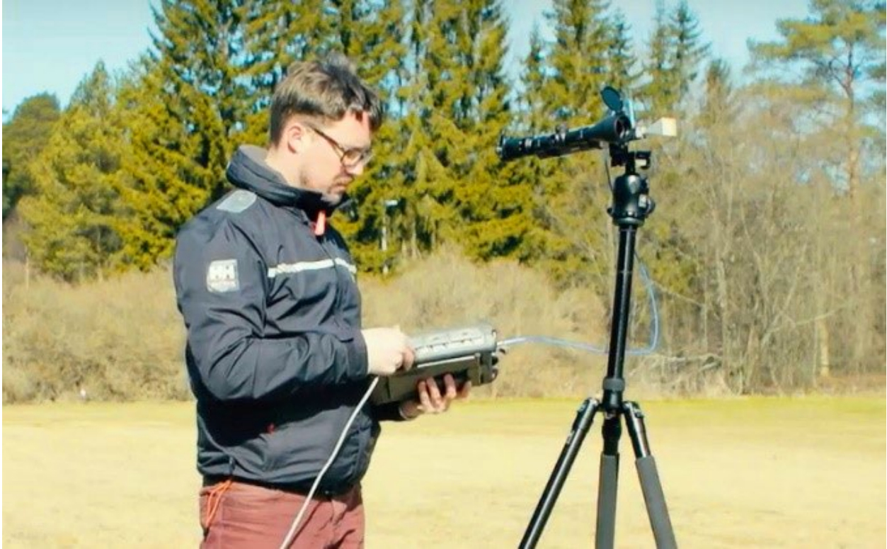
Figure 3. A 54 GHz FieldFox with horn antenna acts as a receiver to measure satellite ground station path loss
