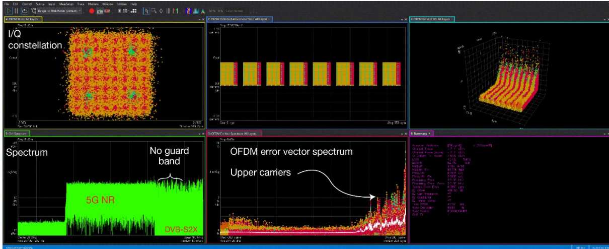
Figure 6. A 28 GHz 5G NR (New Radio) signal interferes with an adjacent satellite communications DVB-S2X digital broadcast and shows degraded modulation analysis metrics
