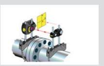
Measurement range may be extended manually in what some might call 'Freeze-frame'. This range extension allows the adjustment of the laser beam such that it does not miss the detector surface when measuring
