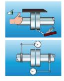
Some misalignment will almost always remain due to low resolution and accuracy. Using the Laser Shaft Alignment tool, a laser is projected onto the reflector mounted on the opposite shaft giving accurate results of all alignment parameters monitored simultaneously. Precision shaft alignment saves energy, time, and makes your machines run smoother and longer.
