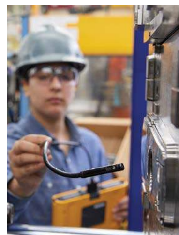
FLK-5.5MM/0.2M ART Articulating Camera FLK-9MM Scope Forward view, 20M probe reel
