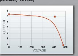
Most often a softer (less square) knee is just the result of the tilting inward of the vertical or horizontal (or both) legs of the I-V curve, deviations 5 & 6. A much less common cause is cell degradation involving a change in the cell ideality factor.
