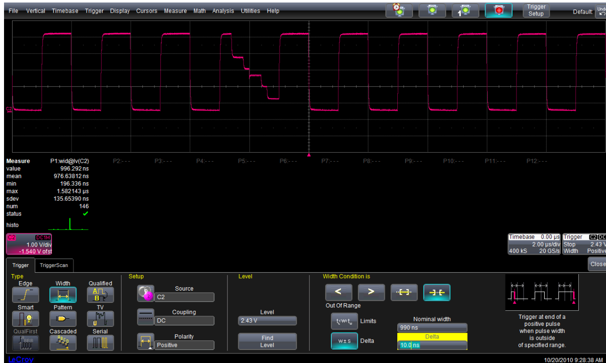
Figure 5: The setup of a SMART Trigger exclusion trigger using pulse width
