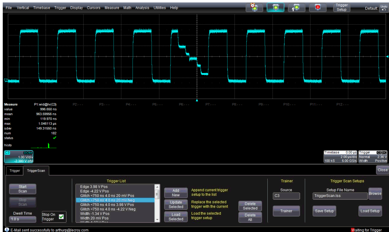
Figure 11: The result of a TriggerScan capture of a glitch. The highlighted entry in the TriggerList shows that the trigger setting used to capture this anomaly was a Glitch trigger with a width <750 ns
