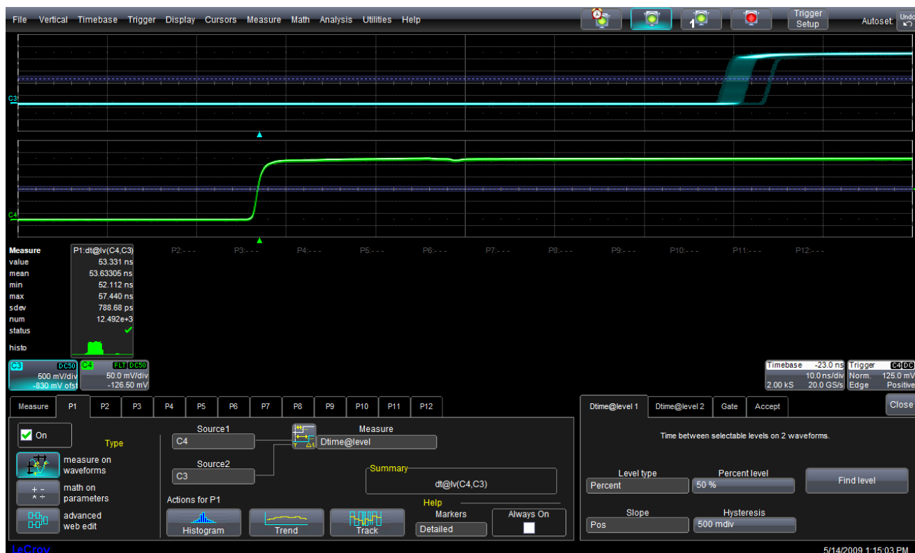
Figure 1: 1 A WaveStream history showing a timing anomaly in a timing synchronizer
