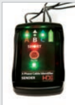
LED lights indicating connected and shorted phases
