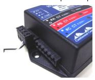
5. Connect Current Transducer(s) to the CT Block on the WattNode.
