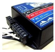
6. Connect Voltage Input Lead Set to the Screw Terminal Block on the WattNode.
