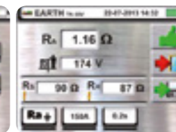
Earth resistance measurement result OK.
