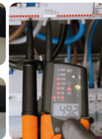
Measurement of phase sequence.
