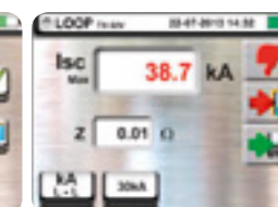
Advanced Loop: negative result of breaking capacity test.
