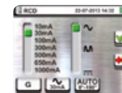
Selection of RCD type and tripping current
