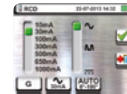
Selection of RCD type and tripping current
