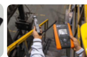
Lux measurement with accessory HT53/05.
