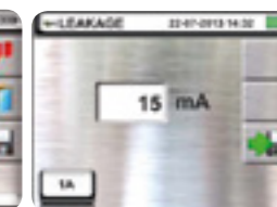
Leakage current with optional clamp 96U
