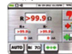
Continuity of protective conductors: Measurement result negative
