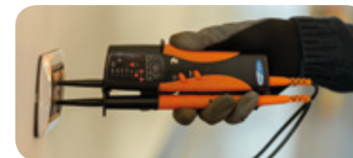
Multimeter function with display and LED indication.
