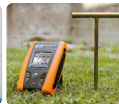
Measurement of earth impedance by voltammetric method
