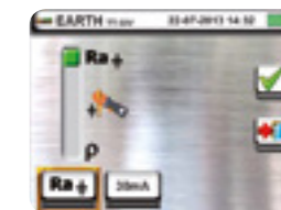
Selection of earth measurement type.
