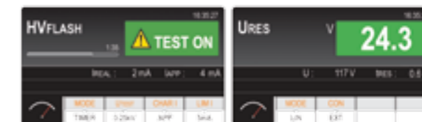
Dielectric strength test
