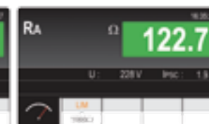
Measurement of non-trip earth resistance
