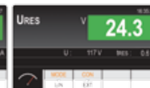
Residual voltage measurement
