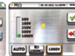
Selection of test voltage and minimum limit value on MΩ measurement
