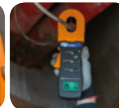
Earth resistance measurement with clamp T2100.
