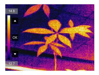
**Note:** Clicking sound and frozen image is a normal phenomenon. The "clicking noise" is generated by FFC(Flat Field Correction), which is used to correct the non-uniformity of the display, improve image quality, and achieve better temperature results.
