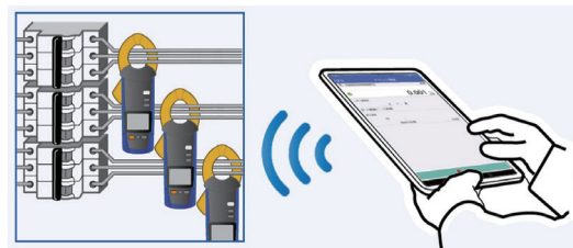
Fig. 16. Setting electric leak thresholds.
