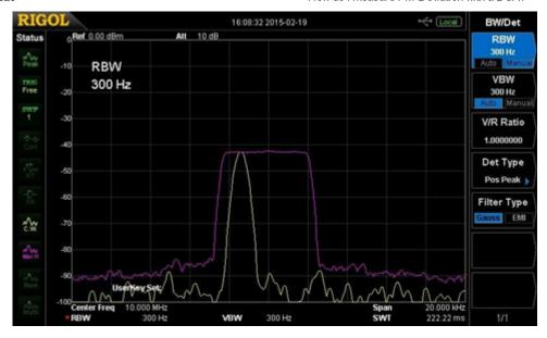
The DSA815 has 10 divisions on the display. The span in this example is 20kHz. So, each division is 2kHz. In this example the FM deviation is approximately 2kHz.
