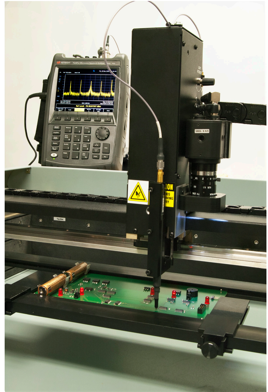
Langer RF-B 3-2 RF Probe fitted to the Access RF Prober. The RF probe is connected to a Keysight N9935A Spectrum Analyzer and is used to measure near field signals on a circuit board.
