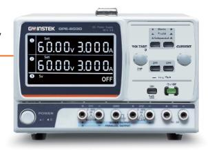
The GPE-3060/6030 are high-resolution linear DC power supplies. Their primary aim is to replace the existing GPC-3060D/6030D models. The GPE-3060/6030 deliver 385 watts of output power and feature three independent isolated output channels. The GPE-3060 offers CH1/CH2 outputs of 0 to 30V and 0 to 6A, while the GPE-6030 supports CH1/CH2 outputs of 0 to 60V and 0 to 3A. Both models feature CH3 outputs of 5.0V at 5A.
