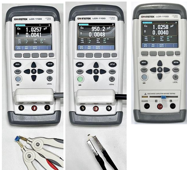
Figure Test results for capacitors
