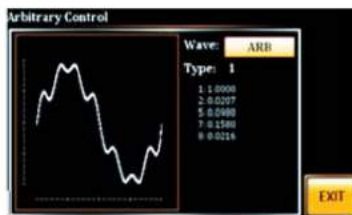
Clipped Sinewave Simulate Grid Power Supply Heavy Load Waveform
