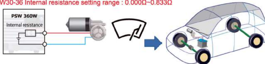
PSW Built-in Resistance Variable Function Simulating Battery Output Resistance and Wire Harness
