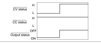
CC MODE: The diagram below shows the timing diagram Output turned on when the output is turned on when the PSU is set to CC mode.
