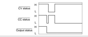
CC MODE: The diagram below shows the output status lines Output turned off when the output is turned off in CC mode.
