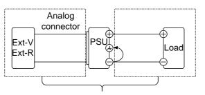
$( \cdots \cdots ) \mbox{ Insulation capacity } \geq \mbox{ voltage of power } supply \mbox{ with respect to ground }$
