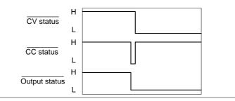
CV MODE: The diagram below shows the output status lines Output turned off when the output is turned off in CV mode.
