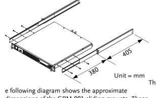
dimensions of the GRM-001 sliding mounts. These sliding mounts should only be used within racks with a depth of 500mm.
