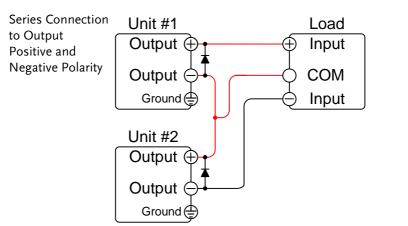
Note: The output reference ground (COMMON) can be grounded at the power supply side instead of the load, depending on the requirements. Local sensing should be used in this configuration.
