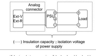
WARNING If the insulation capacity of the load and load cables are not greater than the isolation voltage of the power supply, electric shock may occur. Grounded output If the positive or negative terminal is connected to terminal If the protective ground terminal, the insulation capacity needed for the load and load cables is greatly reduced. The insulation capacity only needs to be greater than the maximum output voltage of the power supply with respect to ground.
