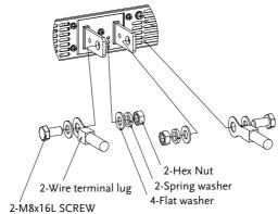
(PSU 100-15, 150- Simply secure the stripped connectors inside each 10, 300-5, 400-3.8, terminal. 600-2.6)
